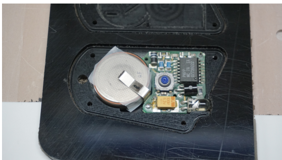
Fig. 4 Test joining of the electronics in the not yet finished component on the CNC milling machine.
