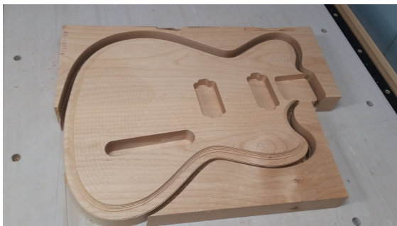
Fig. 3 Production of a guitar body on the CNC milling machine – milled from two sides.
