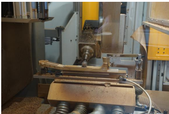
Figure 3 Milling of a guitar neck
