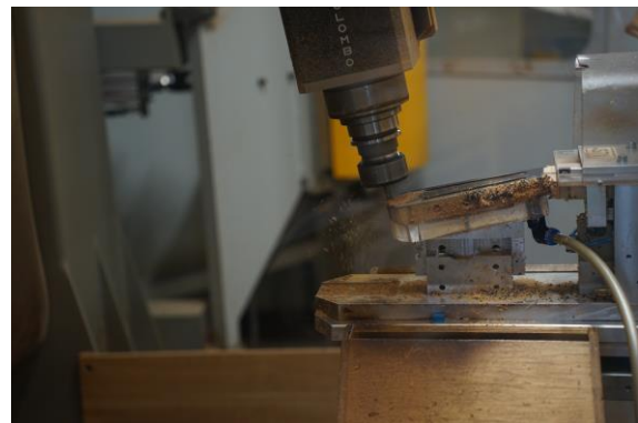
Figure 4 Milling of a guitar head
