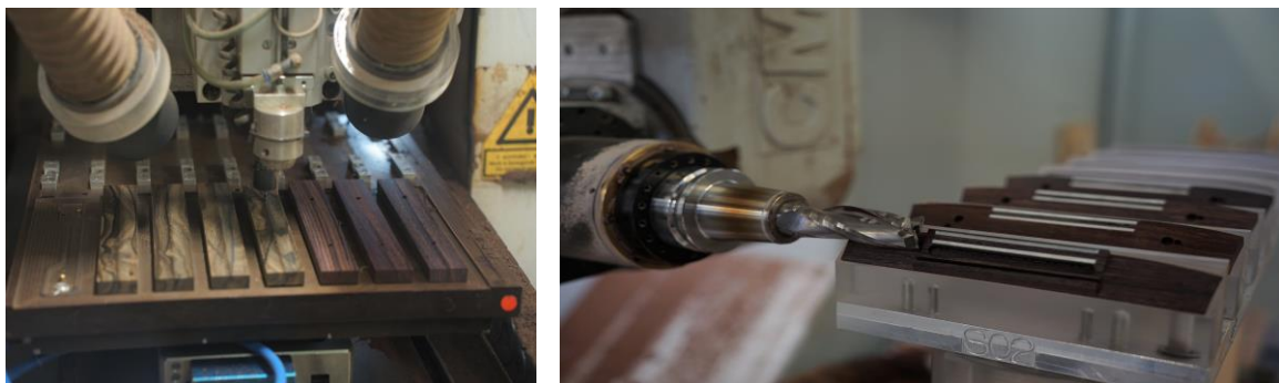
Figure 9 Pre-milling with 3-axis-CNC, final processing of 5-axis-CNC
